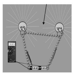
9. Move the <u>right</u> prong so it is on the wire in between the 2 bulbs. What happened to the voltmeter reading? *Why do you suppose this happened*?
