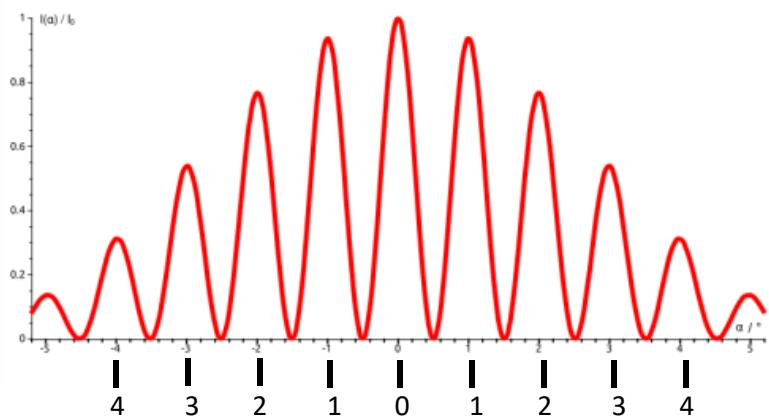
**Rayleigh's Criterion for resolution:** Special case with two light emitting sources upon a single slit.
