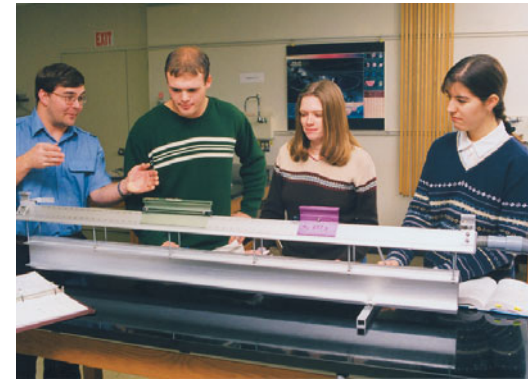
▲ An air track provides a nearly frictionless environment for experiments involving linear motion.
