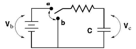
Refer figure above. When the switch is turned on by bringing it to position "a", resister gets connected to  $+V_b$  of the battery. Current starts flowing out of the  $+V_b$  terminal of the battery, flows through R and C, and enters back in  $-V_b$  terminal of the battery. In this process, capacitor gets charged with resistor side of the capacitor becoming positive.
