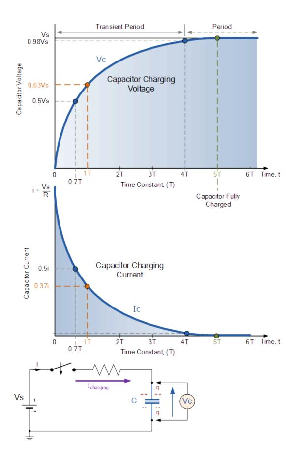
Let us assume above, that the capacitor, C is fully "discharged" and the switch (S) is fully open. These are the initial conditions of the circuit, then t = 0, i = 0 and q = 0. When the switch is closed the time begins at t = 0 and current begins to flow into the capacitor via the resistor.
