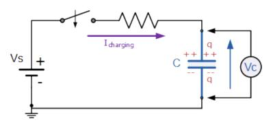
All Electrical or Electronic circuits or systems suffer from some form of "time-delay" between its input and output, when a signal or voltage, either continuous, (DC) or alternating (AC) is firstly applied to it. This delay is generally known as the **time delay** or **Time Constant** of the circuit and it is the time response of the circuit when a step voltage or signal is firstly applied.
