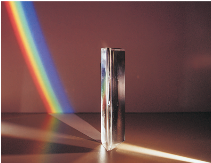
FIGURE 28.2 ▲ When sunlight passes through a prism, it separates into a spectrum of all the colors of the rainbow.
