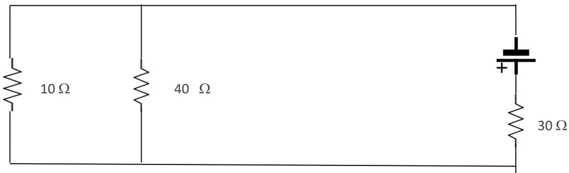
41. If the current in the  $10\ \Omega$  resistor is  $1.0\ \text{Amp}$ , the current in the  $40\ \Omega$  resistor is:
