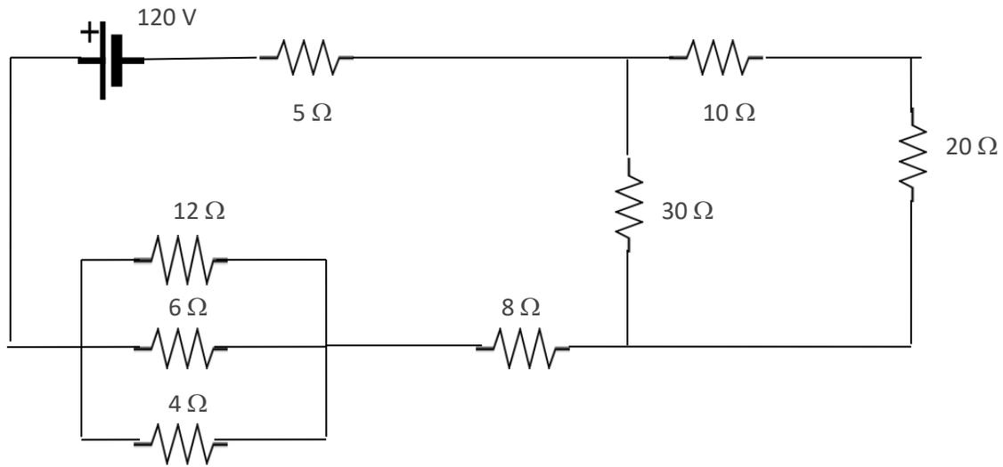
44. Calculate the total resistance in the previous circuit:
