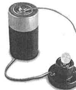
FIGURE 34.3 ▲ Each coulomb of charge that is made to flow in a circuit that connects the terminals of this 1.5-volt flashlight is energized with 1.5 joules.
