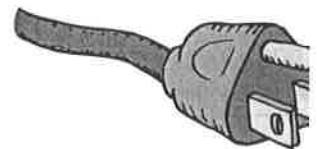
FIGURE 34.9 ▼ The third prong connects the body of the appliance directly to ground. Any charge that builds up on a appliance is therefore conducted to the ground.
