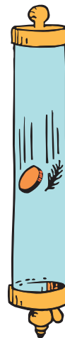
FIGURE 4.13 ▲ A feather and a coin accelerate equally when there is no air around them.
