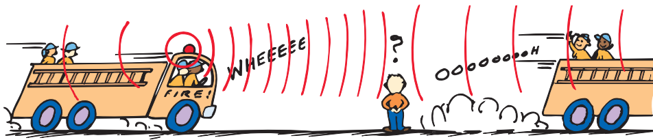
◀ FIGURE 25.17 The pitch of sound is higher when the source moves toward you, and lower when the source moves away.
