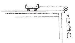
c. Find the acceleration of the 1-kg cart when four identical 10-N weights (not shown) are attached to the string.
