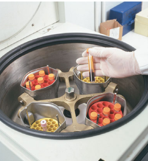
▲ A laboratory centrifuge of the kind commonly used to separate blood components.
