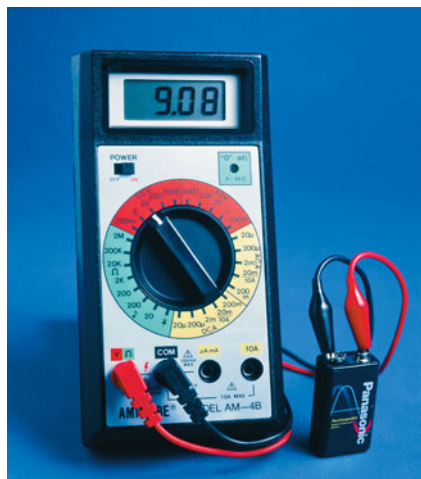
▲ A typical digital multimeter, which can measure resistance (teal settings), current (yellow settings), or voltage (red settings). This meter is measuring the voltage of a “9 volt” battery.
