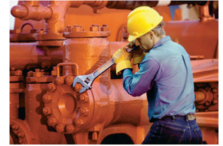
▲ The long handle of this wrench enables the user to produce a large torque without having to exert a very great force.
