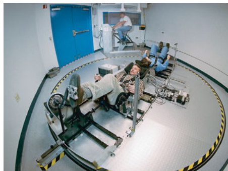
Human-powered centrifuge, designed to give astronauts exercise and artificial gravity during long space flights.
