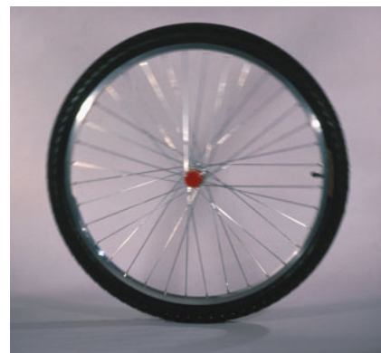
▲ This photograph of a rolling wheel gives a visual indication of the speed of its various parts. The bottom of the wheel is at rest at any instant, so the image there is sharp. The top of the wheel has the greatest speed, and the image there shows the most blurring. (Compare Figure 10-11 .)
