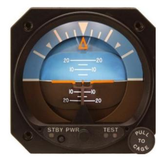
The attitude indicator shows an artificial horizon so a pilot knows that attitude of his aircraft. Both pitch and bank information is shown with the AI. Here the orange bars show the position of the airplanes wings relative to the ground. This intrument is operated from the vacuum pump. If the vacuum pump fails, this instrument will no longer work.
