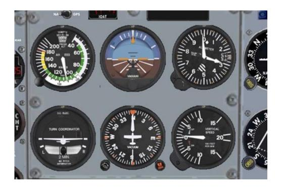
These six primary flight instruments are located together so a pilot can look at them easily. In all modern aircraft, they are in the same positions on an instrument panel, so a pilot will be used to having them in the same position in any aircraft.
